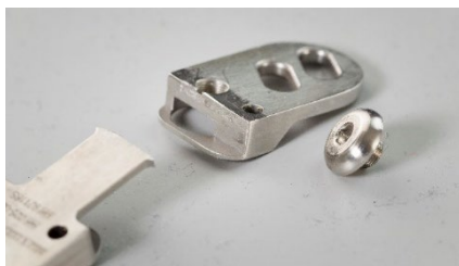
Figure 1. Fractured stabilizer ex vivo
