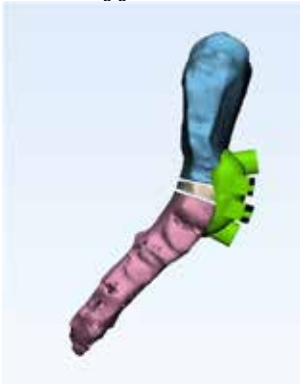
Sideview of sternum and simulated cutting guide in place (green color) 3D printed cutting guide in place
